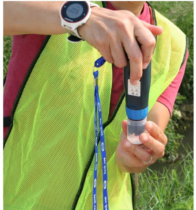
Finally, we received a grant from the Regional Development Authority, and with these funds were able to purchase a Hach Colorimeter. This meter provides much more accurate readings for orthophosphate levels than our previous method of in-field color comparators.
